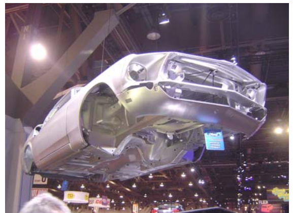
1969 Dynacorn body in white suspended above the 1970 Mustang Sportroof shown below.
