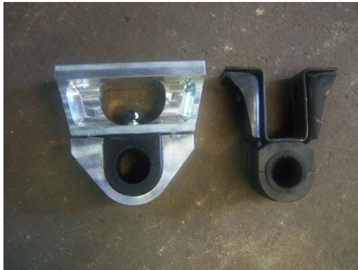
Comparison of the SN95 greaseable Steeda sway bar bracket to the OEM bracket.
