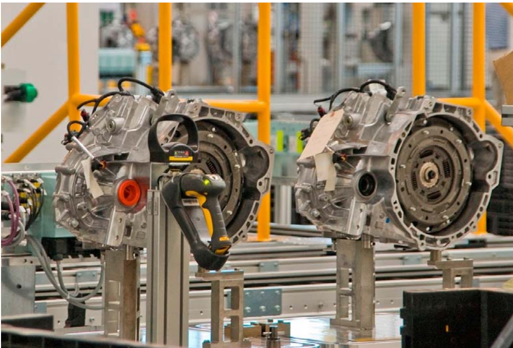
DryDCT transmissions for the Fiesta on the assembly line.
