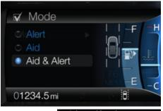
Lane assist is accessed in the lefthand cluster display using the left-hand five-way steering
